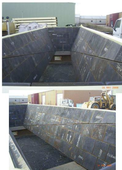
Cadia High Grade Stock Pile Bath Liners supplied in ENDURA Replaced Ni Hard – 2008 Replaced in 2012 after 4 years in service . ENDURA Dual 50 mm upgrade liner material Proposed for this application at Cadia Mine .
