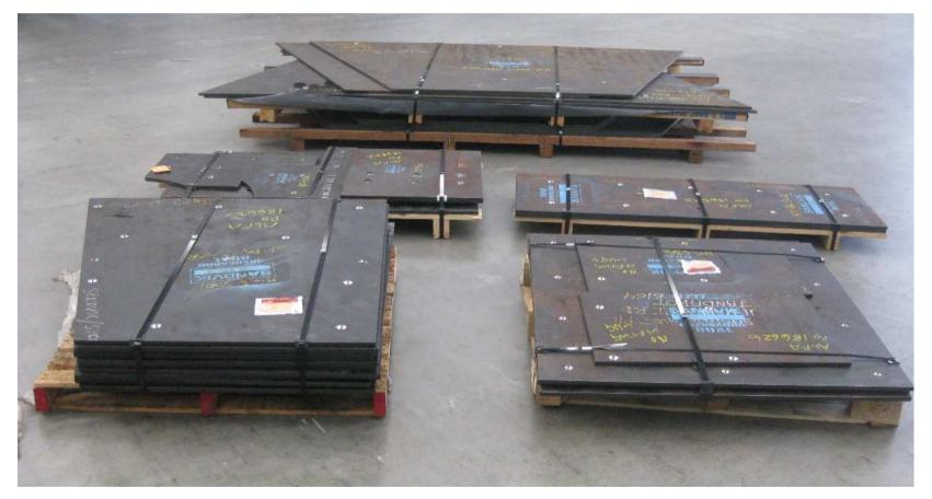
The NEW Standard Approved and Ready To GO ENDURA Dual 16 & 20 mm Liners ready for November 2013 Pilbara mine Fixed Plant Shut down.
