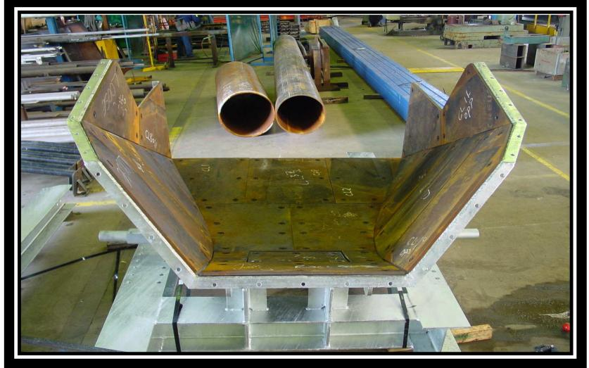
ENDURA Dual Lined Coal chutes –Replacing 450 HB Q & T wear plate Weld overlay has edge wear issues
