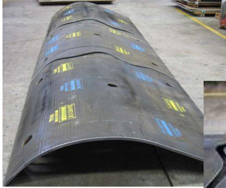
Worlds BIGGEST Loader Bucket liner formed in ENDURA Dual 20 mm 1700 x 6600 mtrs . Supply to Cape Preston - 2009 Replacing Weld Overlay Summary -Selecting the right target to start is important
