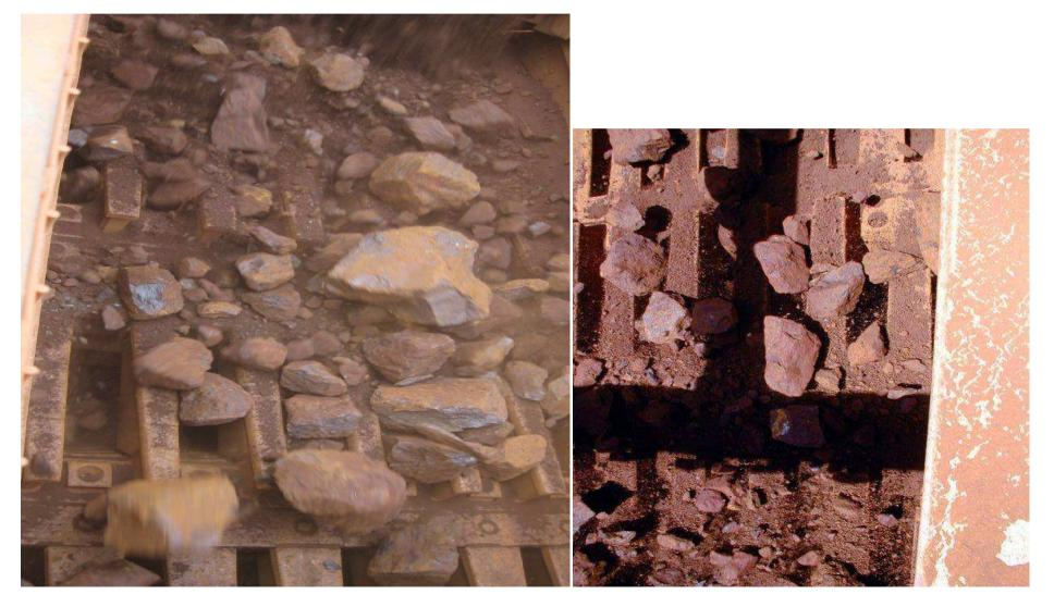
The Grizzle Deck is used to separate lump ore from the fines prior to the primary crusher circuit – Demanding Service Application
