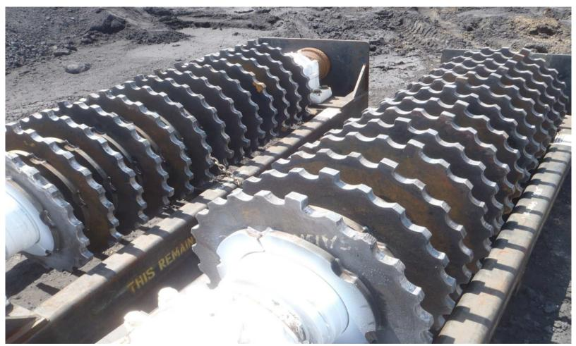
**Coal -25 mm Roller Feeder Screen.** ENDURA Dual FLOWERS Double the Service Life Replacing 500HB Material with hard faced teeth
