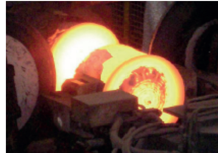
Rotating knives in blanks manufacturing, Toolox 44.
